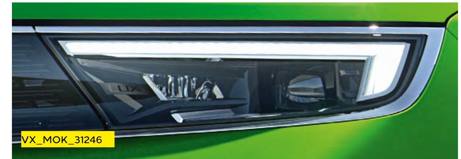
IntelliLux adaptive LED® Matrix headlights.
