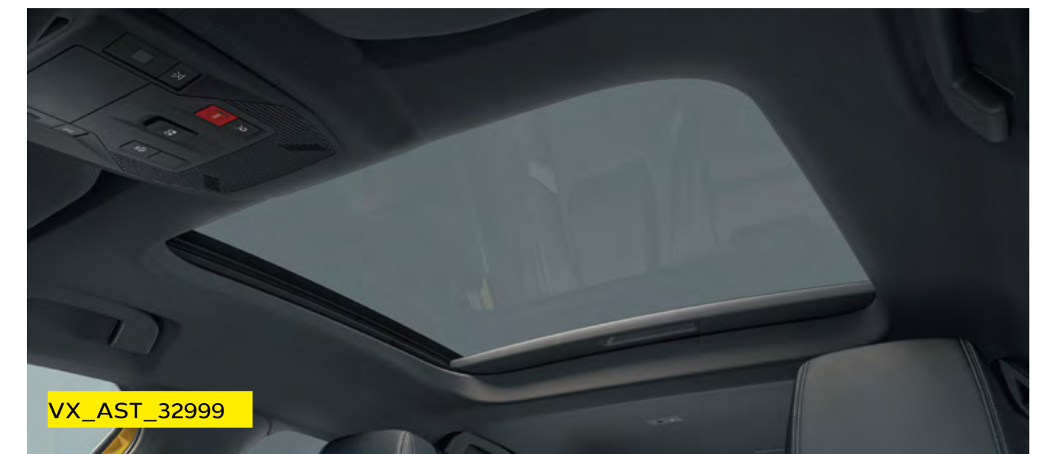
Electrically operated slide/tilt glass sunroof with blind.
