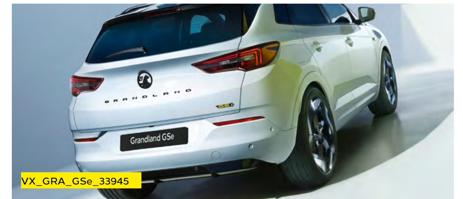
VX_GRA_GSe_33945 GSe rear protective skid plate.
